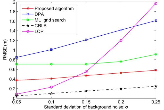
Fig. 8. Comparisons in accuracy as noise standard deviation changes through 5000 trails for a fixed sensor configuration.
