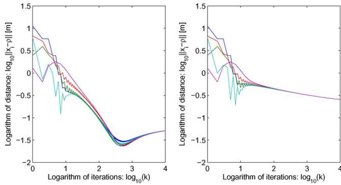
Fig. 3. Estimation errors by proposed algorithm (6) (left) and the DPA in [12] (right) in the inconsistent case.
