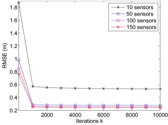
Fig. 10. Estimation errors by proposed algorithm (6) for four different number of sensors.
