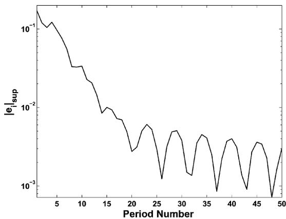
Fig. 3. Error convergence using periodic adaptation (constant  $b$ ).
