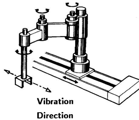
Fig. 1. A SCARA robot with a long tip arm.
