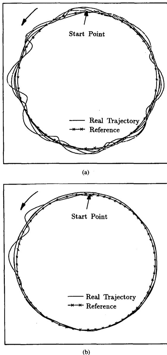
Fig. 9. Traces of end-effector for a circular trajectory: (a) without shear force feedback; (b) with shear force feedback.
