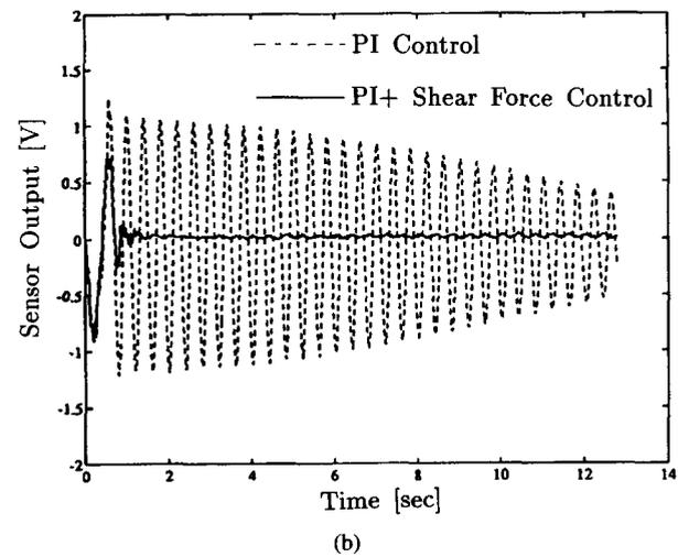
Fig. 6. Time responses of the outputs of shear force sensor: (a) sensor output along the X-direction; (b) sensor output along the Y-direction.
