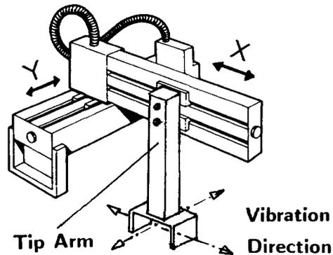
Fig. 2. A Cartesian robot with a long tip arm.
