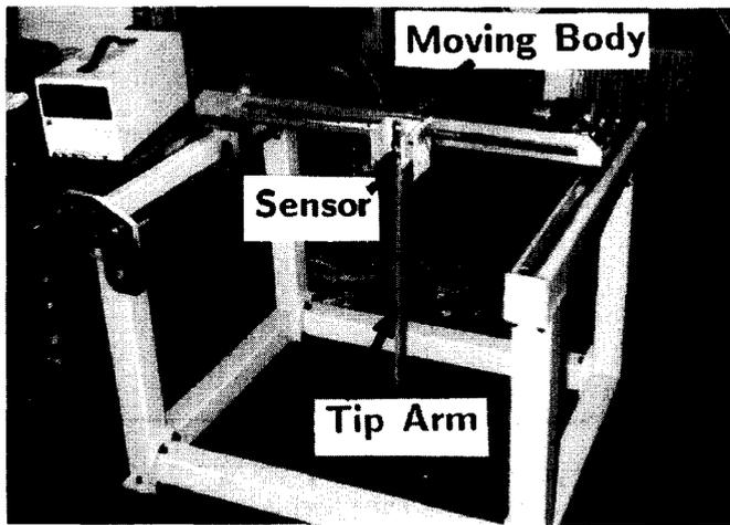
Fig. 5. An X-Y Cartesian robot used for experiments.
