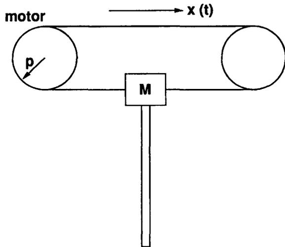
Fig. 4. An illustration of transformation from rotational motion to linear motion via timing belt.
