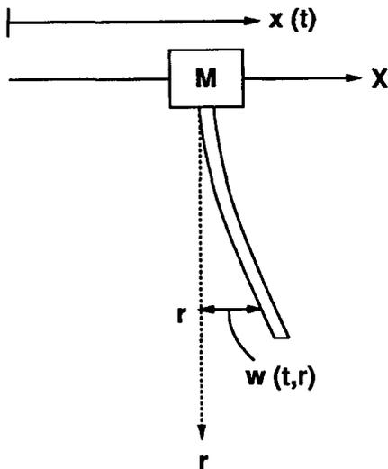
Fig. 3. Vibration of the tip flexible arm of a Cartesian robot along the  $X$ -axis.
