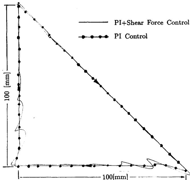
Fig. 10. Traces of end-effector for a trigonometric trajectory. The real line represents trace without shear force feedback; the line with dot marks represents trace with shear force feedback.
